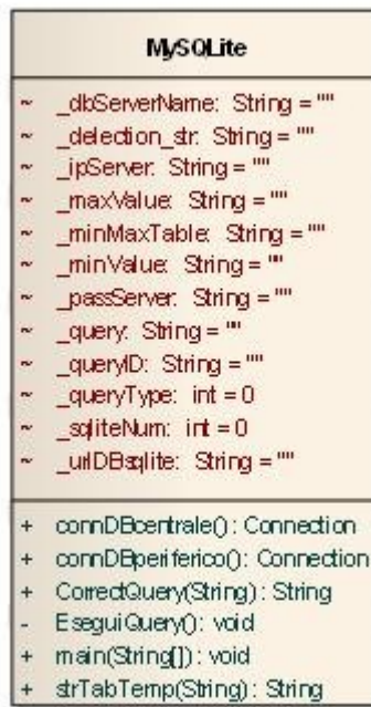
Figura 26 - Remote Module - Class Diagram
